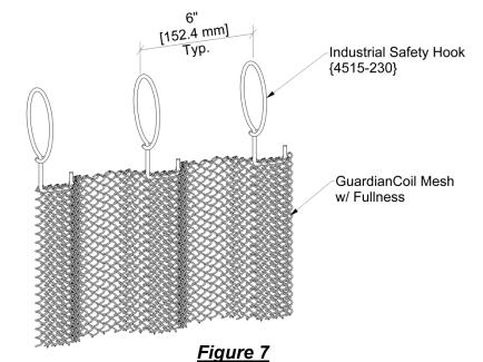
**Step 1:** Bunch 4-5 Mesh Coils together at the Hook location.
