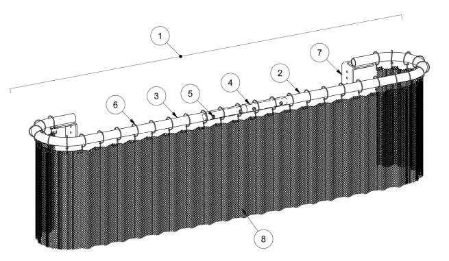
Note: The Vertical Mounting Kit allows the Press Guard Assembly to be installed on the *front* or the *side* of the press frame. (Side configuration shown)
